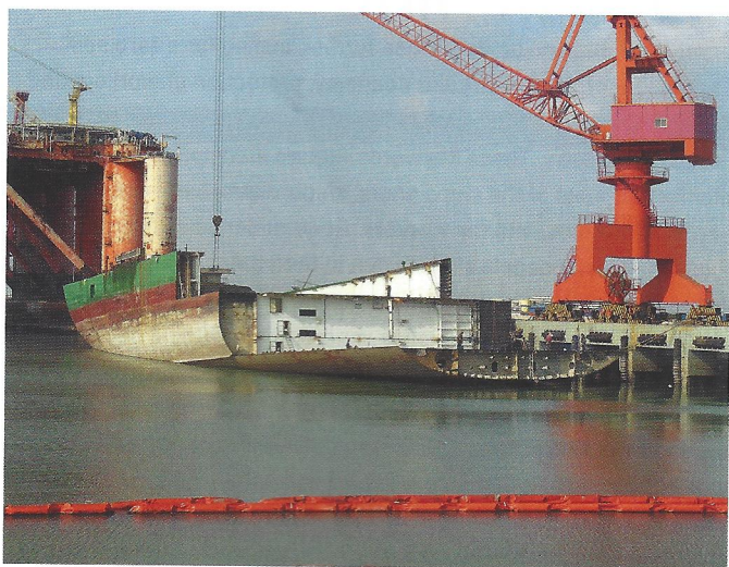
Aft trimmed hull section as fluids containment. Note the oil boom in place and the crane used for controlled recycling (courtesy Sea2Cradle).
