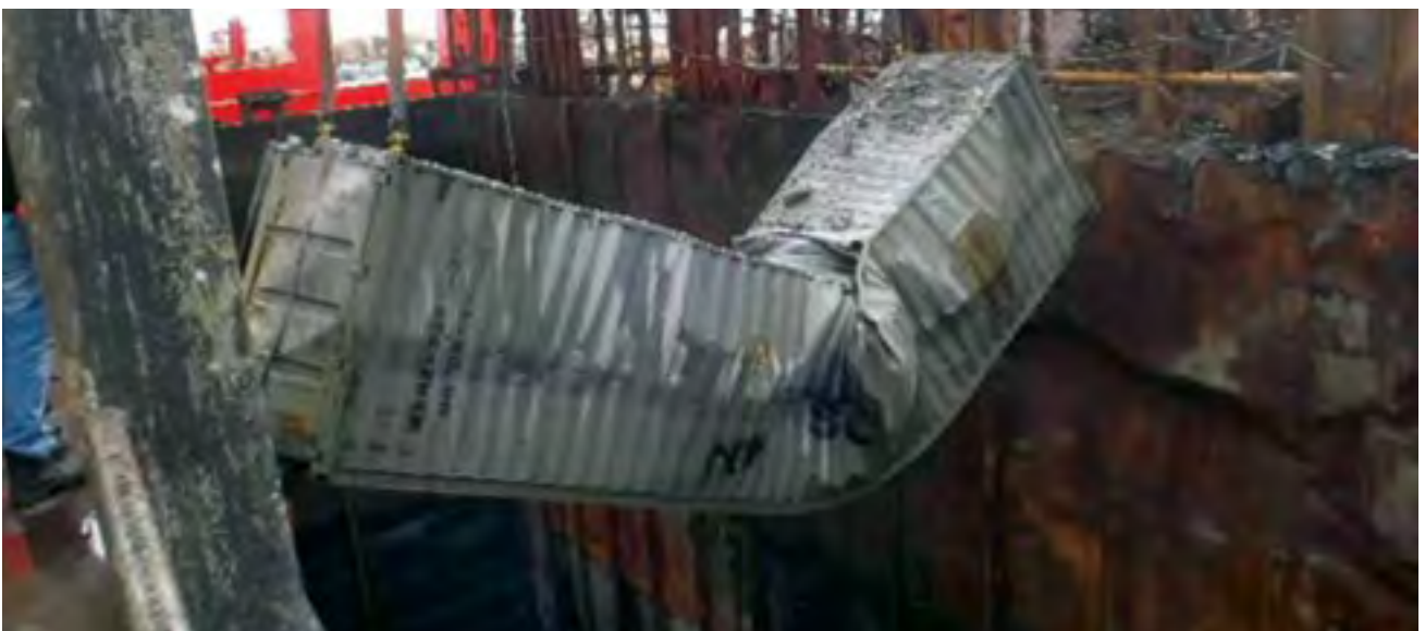
Containers that have been submerged for several weeks may have their longitudinal strength compromised and may bend upon lifting
