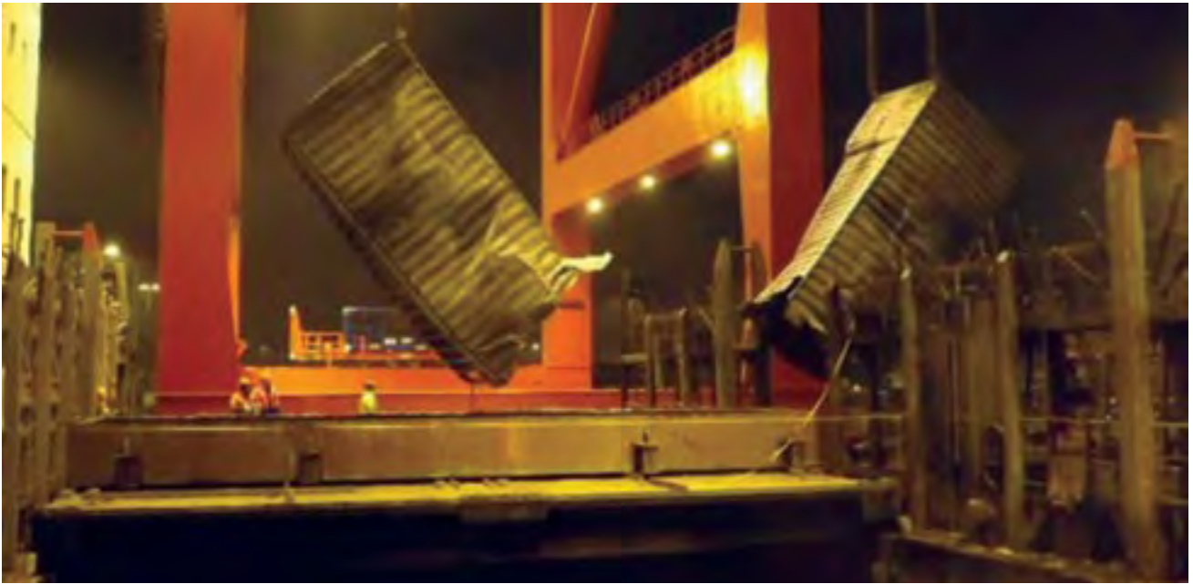
Containers stuffed with cargoes that have absorbed water will have their weight considerably increased and may break upon lifting, with cargo falling into the holds
