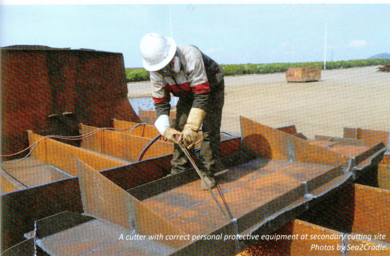
Blocks at secondary cutting site awaiting to be cut into smaller pieces
